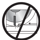
NO CHIPS BETWEEN CUTTER AND SUBSTRATE
