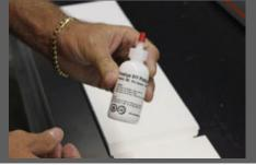
Apply PVC adhesive to one half of each miter.
