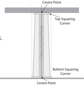
**3.** Once the positions of the squaring corners have been measured and marked, fasten one top squaring corner into the pre-determined position.
