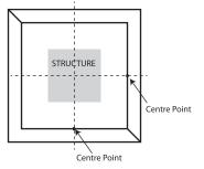
c) Run a level line from the center mark of the bottom squaring corner of both adjacent sides to the top of the beam where the top squaring corner will be positioned.
