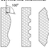
Use a fine-tooth hand saw or power saw with a combination blade. Cut into the exposed face of the material. Use only carbide-tipped or diamond-tipped blades with Extira panels. To produce decorative applications, rout, groove or machine Extira panels. The routed or grooved product should not have any surfaces where water can accumulate. Maintain an angle of at least 100 degrees from the vertical
