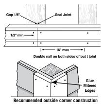
cut end of Extira panels. For fascia, Extira panels must be double nailed and fastened a maximum 24 inches-on-center. For all other applications, double nail 16" on center.
