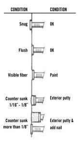
Tapered or bugle head fasteners are permitted when the heads are properly sealed from moisture.
